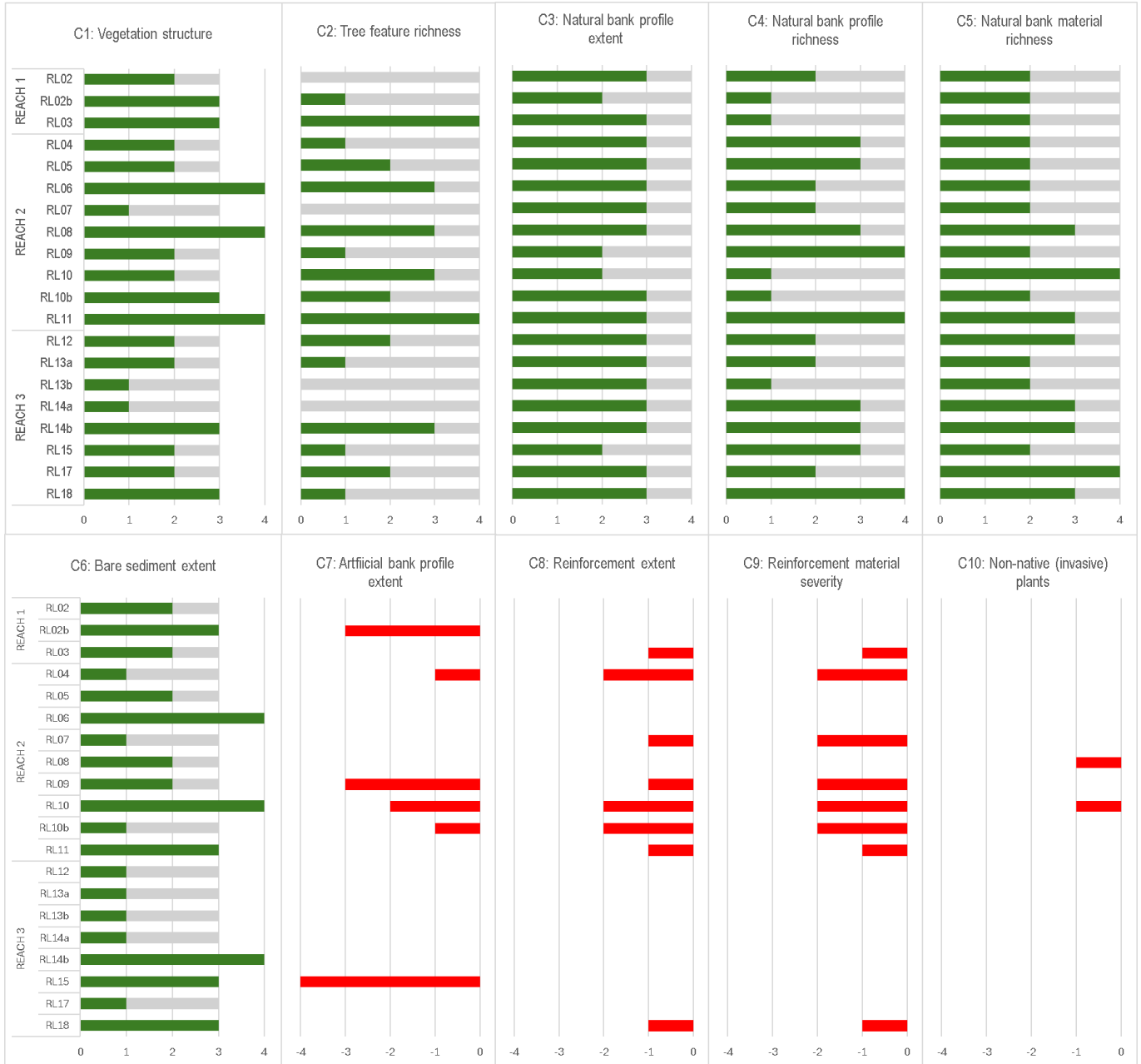
Figure 5: Charts showing the positive (green bars) and negative (red bars) indicator scores for the bank face across each of the surveyed subreaches. Grey bars show maximum expected positive score for the river type.
